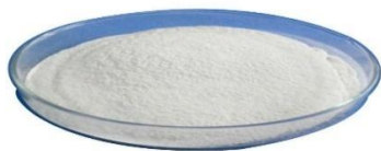
Figure 2. Carboxymethyl cellulose bio-polymer.
