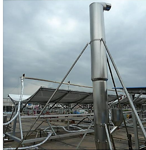
Figure 1. An illustration of a cut tobacco drying system using a parabolic trough concentrating solar heating [44]
