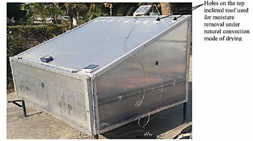
Figure 6. An illustration of the MRT solar cabinet dryer with the reflector sheet on the north wall [49]
