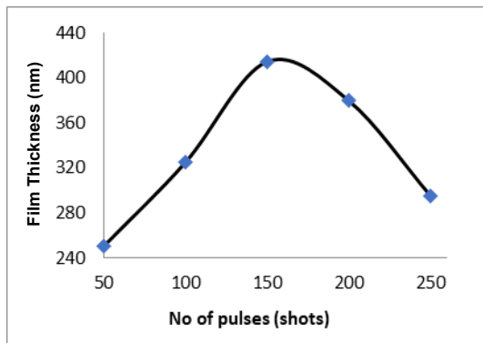
Figure 4. Film thickness versus Number of pulses of \text{Al}_2\text{O}_3 nanostructures
