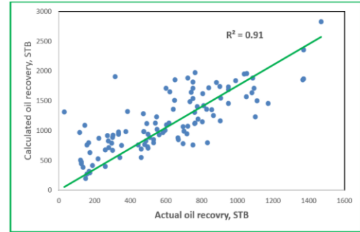
Figure 6. Cross plot for oil recovery (API correlation).
